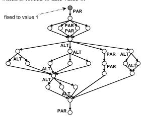
Fig. 2. Example of P/A graph with PAR/ALT annotation.
