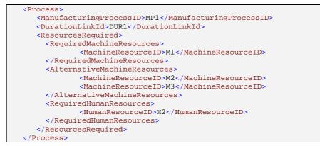
Fig. 3. Description of Machine and Labor Requirements for a Process.
