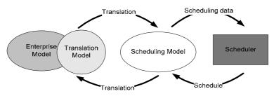
Fig. 1. Integration Architecture between Enterprise Model and Scheduling model.
